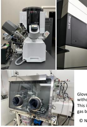
Left: The latest plasma FIB sample processing observation device. Observe, analyze and process asteroids samples. Right: A scanning transmission electron microscope used to investigate the kind of substances Ryugu is made from.
