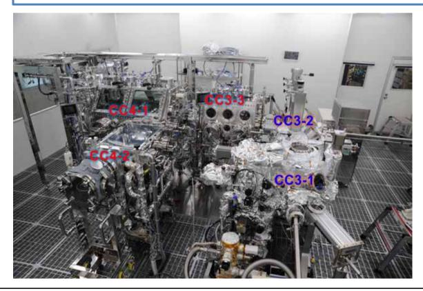
CC3-1 : Opening the sample container under vacuum environment CC3-2 : Sample collection under vacuum CC3-3 : Transition from vacuum to nitrogen environment CC4-1 : Handling of submillimeter-sized particles CC4-2 : Handling / observation / sorting of relatively large particles (> mm)
