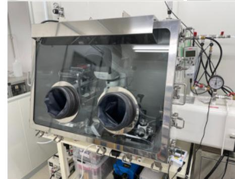
Glove box for handling samples without exposure to the atmosphere. This is filled with purified nitrogen gas before use.
