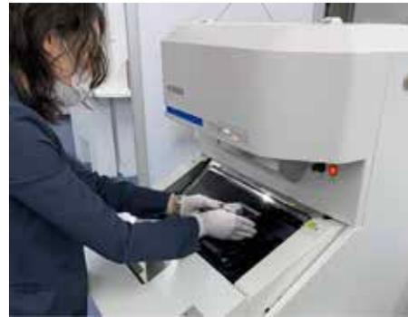
Thermal ionization mass spectrometer for isotope analysis and dating (© Tokyo Institute of Technology)
