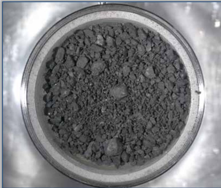
Optical microscope image of the chamber A sample (before individual particle selection)
