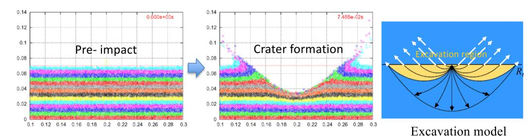
An example of numerical simulations of crater formation impacts on a granular layer (sand). Color corresponds to the depth prior to collision. (Provided by Koji Wada)
