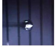
② Projectile shape Observed flight speed is 2km/s. The outer diameter is about 135mm and weight 2kg. The shape is like a helmet.
