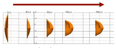
Copper plate (liner) that deforms as it flies
