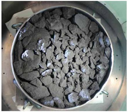
Target simulating the surface of Ryugu. (image credit: JAXA, University of Tokyo)
