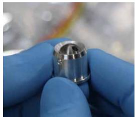
Projector (barrel) and projectile (bullet) used: as these are flight spares, the shape, material etc are the same as those onboard Hayabusa2. (image credit: JAXA)
