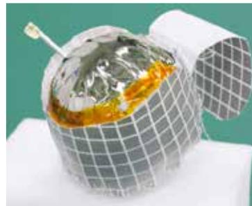
The target marker is placed within the reflective sheet and sewn with yarn so there are no gaps.
