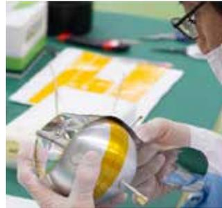
The films are wrapped around the ball-shaped core of the target marker.
